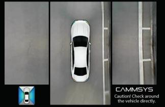
Vehicle indicators on - turning left/right: When the indicators are used, the system can project the left and right camera images onto the screen in addition to the top view, providing the driver with a perfect view of objects close to the vehicle. This prevents kerb damage to wheels and hitting low objects which are in your blind spot.
